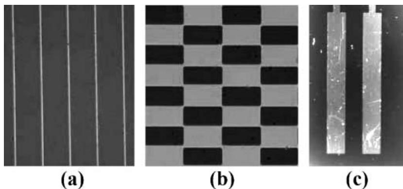
**Figure 1.** Photomicrographs of patterned chips used in this study: (a) parallel gold lines (20  $\mu\text{m}$  wide lines separated by 500  $\mu\text{m}$  spaces) that are connected to a single lead; (b) grid of interconnected gold rectangles (200  $\mu\text{m} \times 360 \mu\text{m}$ ) that are connected to a single lead; (c) chip with two gold rectangular electrodes (8 mm  $\times$  1 mm) that are connected to separate leads (i.e., the electrodes are electrically independent).
