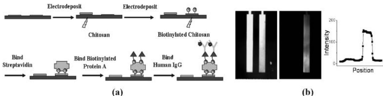
**Figure 4.** Streptavidin-mediated protein assembly: (a) schematic of experiment; (b) bright-field photomicrograph and fluorescence intensity profile showing fluorescently labeled IgG is assembled onto the right electrode (with biotinylated chitosan) with little non-specific assembly on the left electrode (with chitosan).
