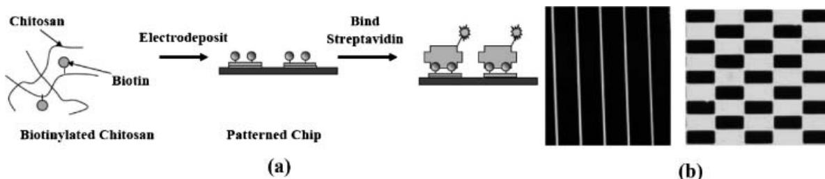
**Figure 2.** Spatially-selective assembly of fluorescently-labeled streptavidin onto patterned chips: (a) schematic of experiment; (b) fluorescence photomicrograph showing fluorescently-labeled streptavidin is assembled onto the patterned electrodes used to electrodeposit biotinylated chitosan.
