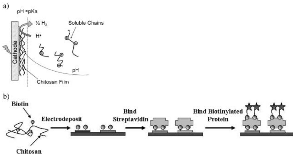
**Scheme 1.** (a) Chitosan can be induced to undergo a localized sol-gel transition in response to the localized pH gradient created by electrochemical proton consumption at a cathode surface; (b) a method for streptavidin-mediated protein assembly.
