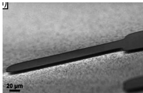
**Fig. 14** Partially released chitosan cantilever on silicon with dimensions  $240 \times 25 \times 2 \mu\text{m}$ . Chitosan serves as a sufficient structural material to support itself. Reprinted with permission from ref. 14. © 2008 IEEE.
