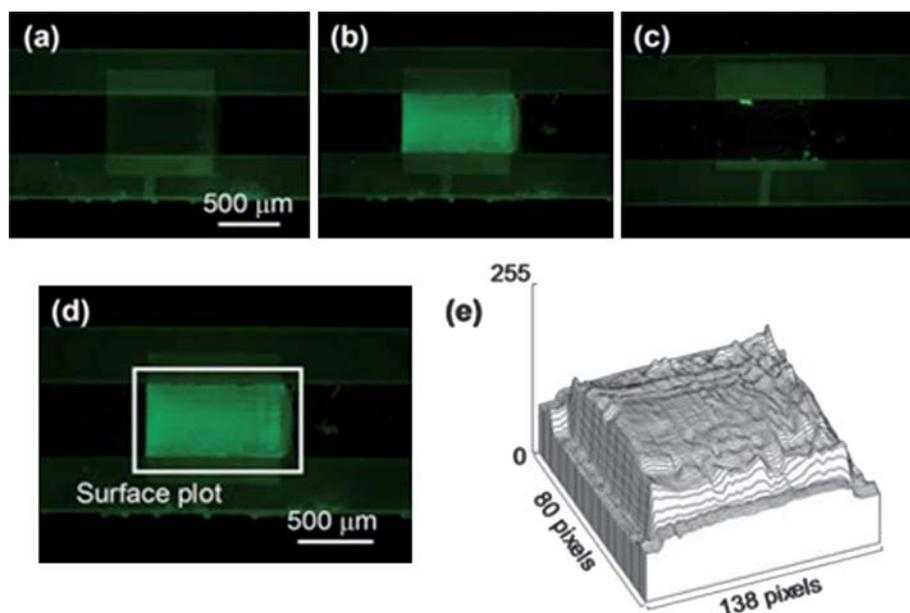
**Fig. 7** Chitosan mediated assembly of GFP in micro fluidic device. (a) Fluorescence image of the assembly site after glutaraldehyde reaction; (b) after GFP reaction; (c) negative control (no bias); (d) GFP conjugated chitosan film; (e) Image J fluorescence surface plot.<sup>57</sup>—Reproduced by permission of the Royal Society of Chemistry.
