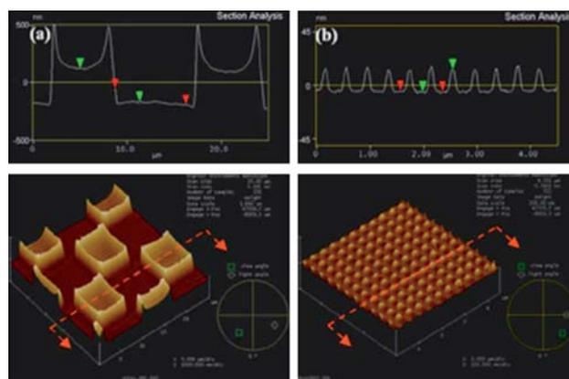
**Fig. 6** Examples of AFM images taken of (a) printed chitosan squares 6.7  $\mu\text{m}$  across and (b) chitosan nanodots with 150 nm width and 400 nm pitch. Reprinted with permission from ref. 13. Copyright 2007, American Institute of Physics.
