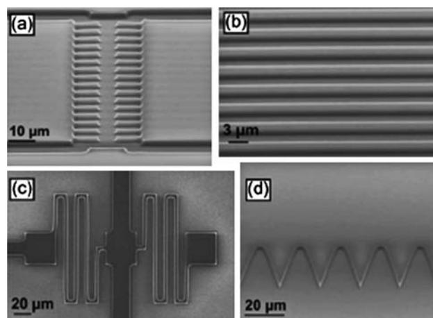
**Fig. 2** Photolithographically patterned chitosan features. (a) SEM of a matched comb structure at a 50° tilt. (b) SEM of 2-μm-wide lines with 4-μm pitch. (c) SEM of serpentine spring structures. (d) SEM of a sawtooth structure. Note: All patterns are in a 2-μm-thick chitosan layer. Reprinted with permission from ref. 14. © 2008 IEEE.
