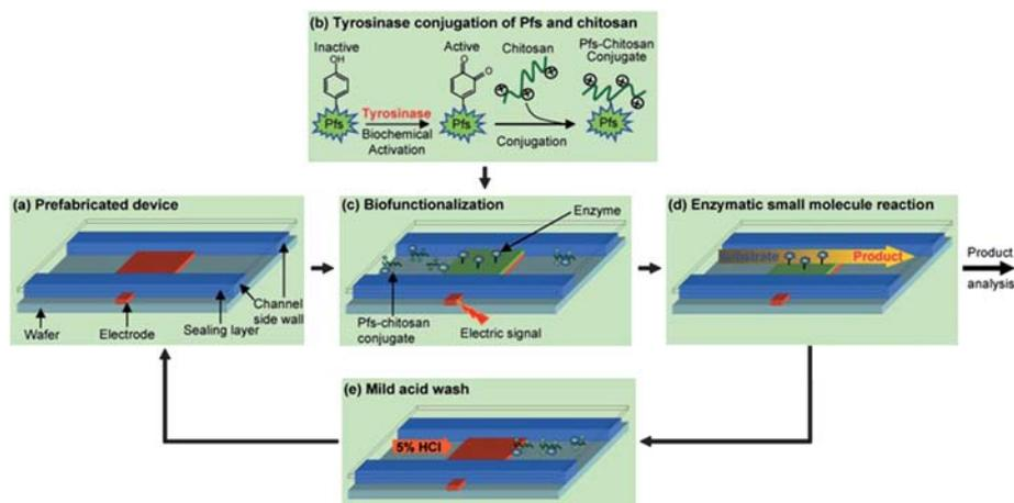
**Fig. 8** Schematic of chitosan conjugation and electrodeposition in a microfluidic channel. (a) Prefabricated device, (b) conjugation between chitosan and the enzyme Pfs, (c) electrodeposition of Pfs-chitosan conjugate, (d) enzymatic small molecule detection, (e) mild acid wash removes chitosan and refreshes electrode surface.<sup>58</sup>—Reproduced by permission of the Royal Society of Chemistry.
