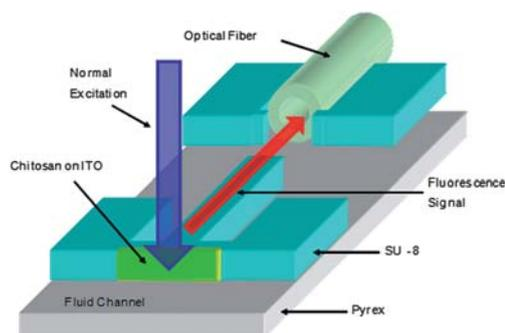
**Fig. 11** Perspective view of optical waveguide sensor with chitosan film on sidewall. The waveguide is shortened to show fiber coupling. The blue arrow represents the optical excitation signal while the red arrow represents the collected fluorescence signal.<sup>20</sup>—Reproduced by permission of the Royal Society of Chemistry.
