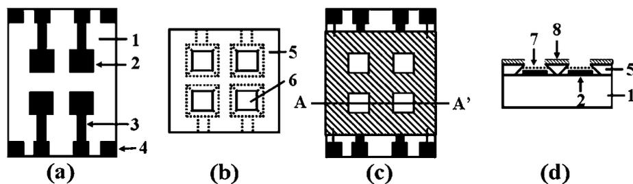
**Fig. 10** Schematic of micromachined amperometric sensor. 1. Pyrex glass down-substrate, 2. Pt WE, 3. Conduction line, 4. Pads, 5. Up-substrate made of silicon, 6. Quadratic hole, 7. Chitosan membrane with cross-linked enzyme, 8. Ag/AgCl RE. (a) Down-substrate, (b) up-substrate, (c) bonding between up- and down-substrates, (d) cross section along A-A'. Redrawn with permission from ref. 24.
