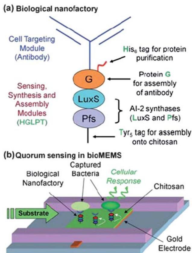
**Fig. 9** Assembly and manipulation of quorum sensing (QS) bacteria in a bioMEMS device *via* biological nanofactories. (a) Components of a biological nanofactory: cell targeting module (antibody); sensing, synthesis and assembly modules (HGLPT nano-construct). (b) The nanofactories are spatially assembled onto chitosan electrodeposited within the device; they capture targeted bacteria and manipulate their QS response.<sup>143</sup>—Reproduced by permission of the Royal Society of Chemistry.
