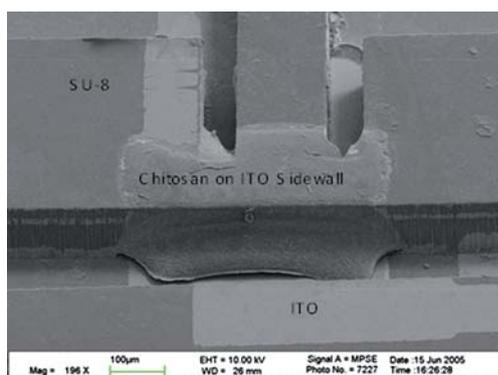
**Fig. 4** SEM of chitosan film electrodeposited on the sidewall of a microchannel. A thin film of patterned indium tin oxide acted as the cathode surface for the deposition. Reprinted with permission from ref. 162.
