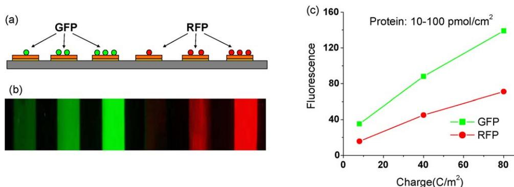
**Fig. 5.** Assembly of two model proteins (GFP and RFP) at individual electrode addresses. (a) Schematic. (b) Fluorescence image. (c) Quantification. Adapted from Shi et al. (2009) copyright Wiley-VCH Verlag GmbH & Co. KGaA. Reproduced with permission.
