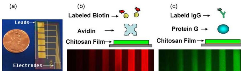
**Fig. 4.** Assembly of avidin and protein G at electrode addresses. Film activation progressively increased from left to right. Visualization was achieved using fluorescence labels.
