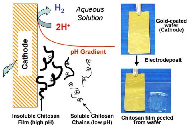
Fig. 2. Chitosan's electrodeposition. Cathodic reactions generate a locally high pH that induces chitosan to undergo a sol–gel transition to form a hydrogel film.
