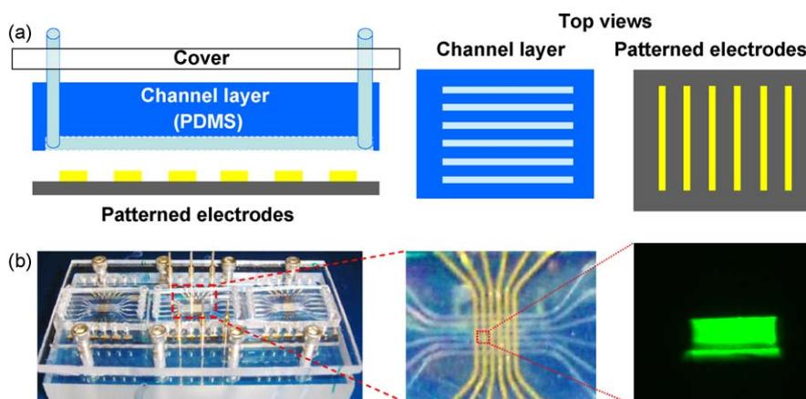
**Fig. 6.** Microfluidic device. (a) Schematic illustrating components of a typical device. (b) Photographs and fluorescence photomicrograph of microfluidic device at various magnifications.
