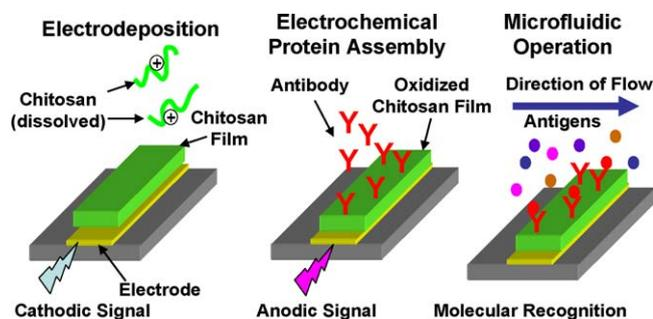
Fig. 1. Schematic illustrating chitosan's potential to interface biological components (e.g., antibodies) to sensor addresses of microfluidic LOCs.
