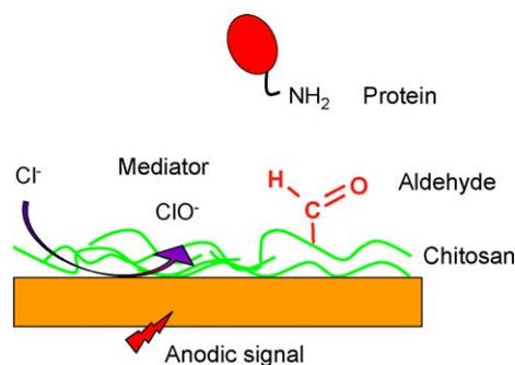
Fig. 3. Proposed mechanism for the anodic activation of chitosan and subsequent protein conjugation.
