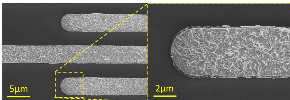
**Figure 6.** SEM images showing the planar symmetric NiO supercapacitor fabricated in the photoresist capillary microfluidic channel. The minimum electrode feature size is  $4\ \mu\text{m}$ .
