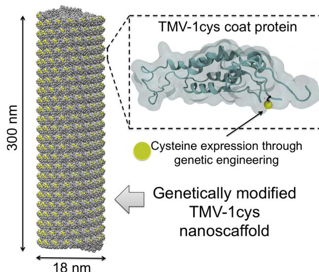
**Figure 1.** Schematics of the genetically modified TMV1cys bionanoscaffold nanorod, and the enlarged view of its CP structures.
