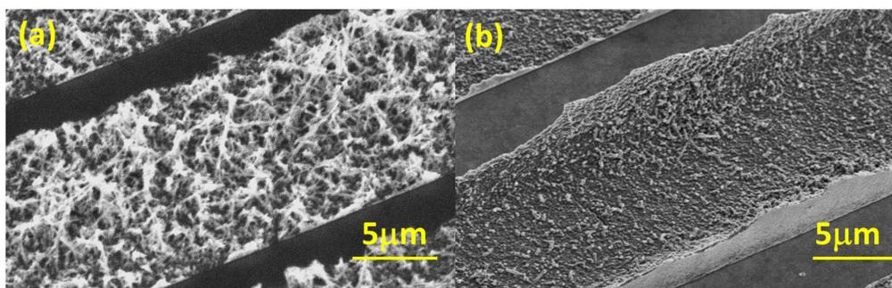
**Figure 4.** SEM images showing TMV nanoscaffolded Ni/NiO electrodes fabricated by evaporation of (a)  $0.2 \text{ mg ml}^{-1}$  and (b)  $2 \text{ mg ml}^{-1}$  of TMVs in capillary microfluidic channels [21].
