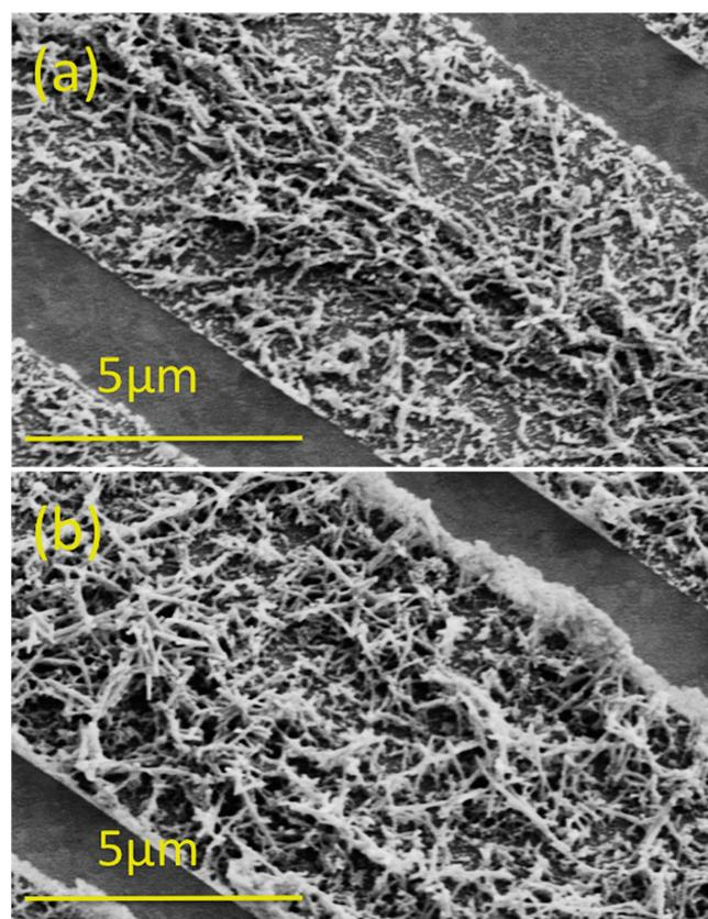
**Figure 5.** SEM images showing the TMV distribution (a) close to the inlet of the channel, and (b) in the center of the microfluidic channel.
