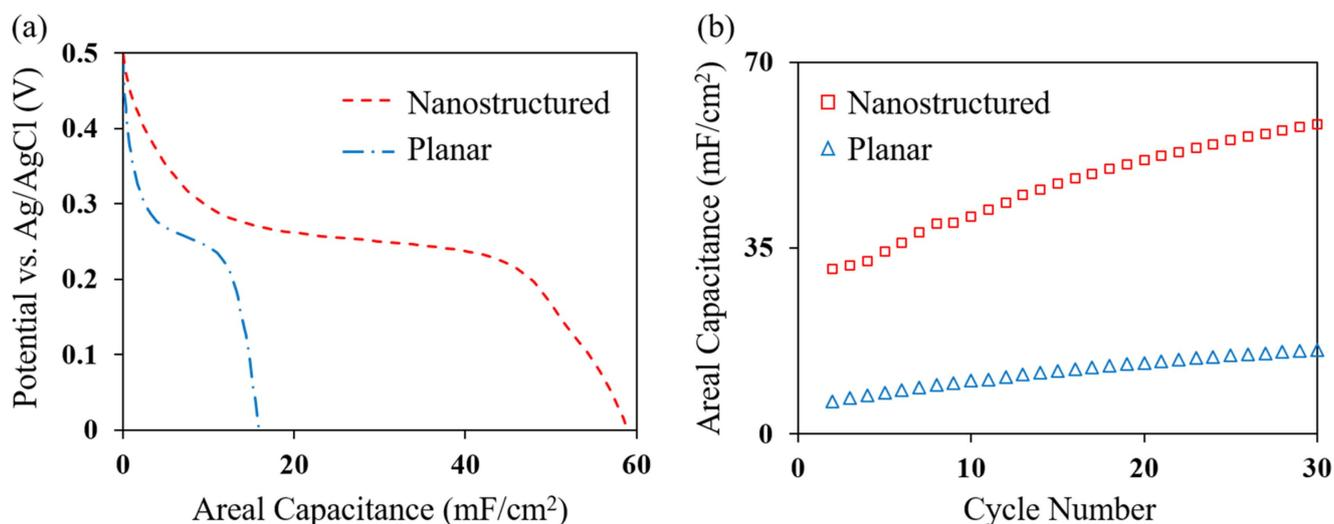
**Figure 7.** Electrochemical characterization of the TMV nanostructured NiO electrodes: (a) comparison of galvanostatic discharge plot and (b) areal capacitance increase by the TMV nanoscaffolds in different cycles.
