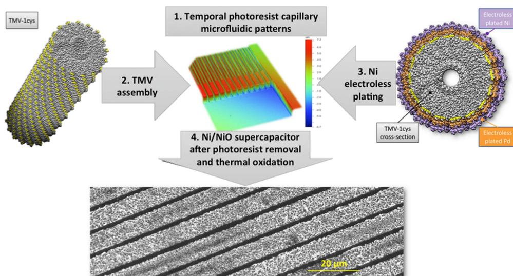
**Figure 3.** Optical profilometry and scanning electron microscopy (SEM) images showing the TMV nanostructured electrode fabricated through coating of TMVs in photoresist capillary microchannels.
