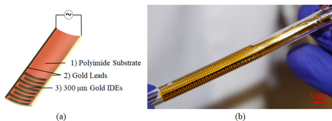
Fig. 2. (a) A schematic of the flexible platform showing 1) the flexible 25.4 \mu\text{m} polyimide substrate, 2) Gold leads for interfacing the sensor with a potentiostat, and 3) Gold IDEs with 300 \mu\text{m} width and spacing over a 10 \times 40 \text{ mm}^2 footprint. (b) An optical image of the device interfaced with the interior lumen of the catheter tube (inner diameter of 4.5 mm). The device is seamlessly integrated onto the curved surface with no signs of degradation, highlighting the advantage of the flexible platform.
